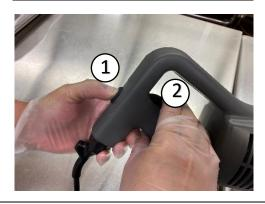
To operate the Immersion Blender, you must first push the safety button at top, then push the trigger in the handle to turn on. Once on, you can let go of safety.
